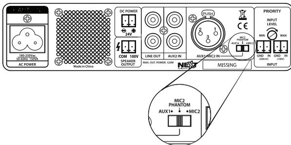
When phantom power is enabled, be careful to choose the right cable for your microphone. It must be a balanced type cable to provide phantom power effectively.
